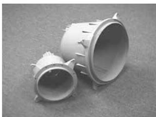
**Gunite Plastic Niches** – These plastic concrete niches are molded of high strength, corrosion resistant PVC with a one inch PVC hub. Both 450 and 3/4 in. reducer bushings are included. Gunite models feature rebar tie-backs and a plaster ring for clean, simple installations and all are packed with a gunite/plaster shield.
